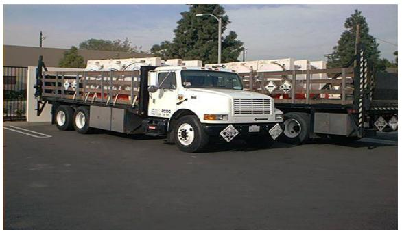
Typical delivery truck. Bulk liquid is pumped from truck to customer's tank via air driven pump. Each delivery is measured and totaled with on-board scale.
