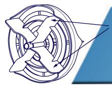
Four fins on both sides of the disc extend fully to engage with adjacent fins, thereby creating a solid wave-retention barrier. No water gets through!
