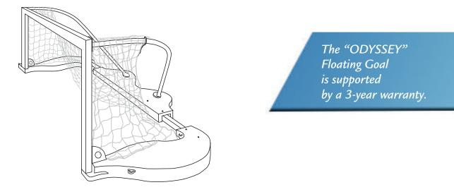
The **"ODYSSEY" GOAL** is a floating water polo goal that was designed for and used in the 2000 Sydney Olympics. It conforms to all **National** and **International** standards. The goal's one-piece welded upright/crossbar assembly, single back brace and two rear struts are all made from white powder-coated aluminum extrusion. Three heavy-duty hand-laid fiberglass floatation panels (two sides and one rear) provide the necessary buoyancy.
