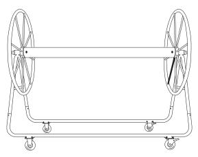
The **Ultimate Storeel** is a high-capacity storage unit for swimming racing lanes. It is of white powder coated, al aluminum construction. The center spool's diameter is 6", designed specifically to minimize damage to the discs when removing lanes from the pool.
