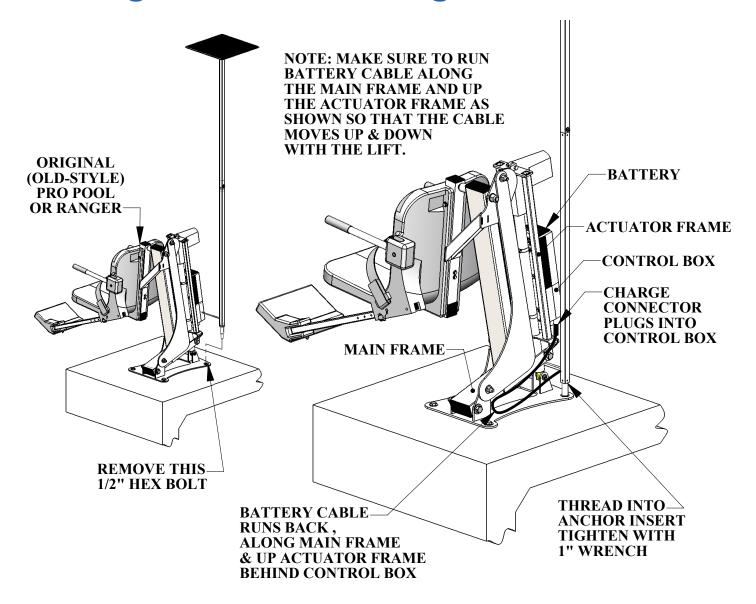
Installing the Solar Charger on an original-style Pro Pool/Ranger Lift;
