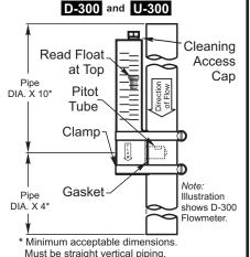
**General:** Flowmeter should only be used on the schedule 40 IPS (ASTM-D-1785) size and type of pipe for which it is intended. Incorrect use will result in inaccurate readings and leakage problems.
