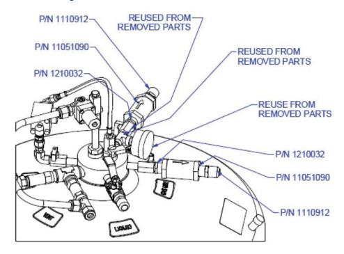
Carbo-Max 750 Bulk CO<sub>2</sub> System Parts to be Removed
