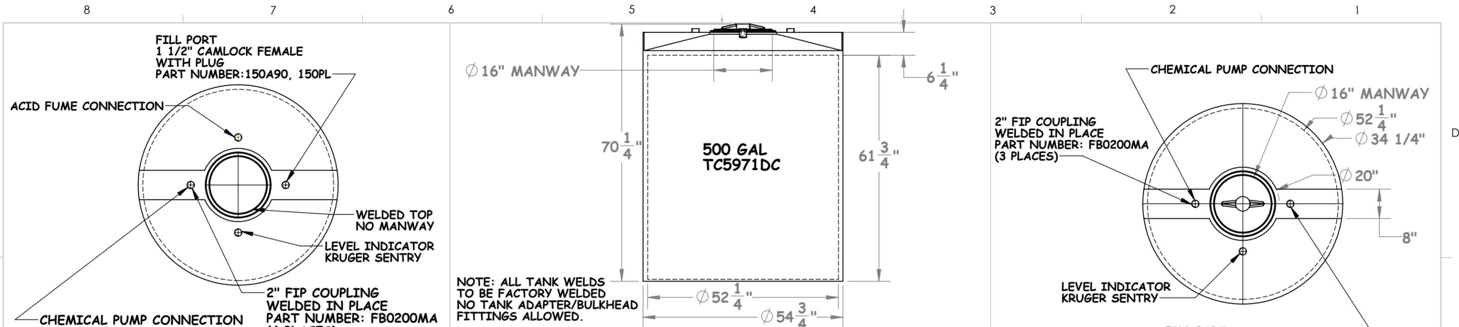
NOTE: ALL TANK WELDS TO BE FACTORY WELDED NO TANK ADAPTER/BULKHEAD FITTINGS ALLOWED.
