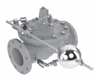
from the control lines and cover chamber. Carefully loosen tube fittings at highest points and bleed air from system. Carefully loosen the plug at top of main valve cover. If an indicator is installed, carefully loosen the vent at top of indicator. If the valve is installed on its side loosen the top 4 cover bolts to bleed air trapped in the cover. Bleed air from cover and tighten plug. Tighten tube fittings.
