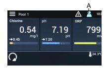
The device offers the option of using up to three user levels. Different rights are assigned to each user level. The colored user symbol (A) in the main menu shows on what level the user is logged in.
