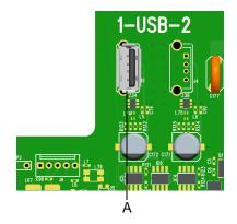
The electronics module is equipped internally with a USB interface. It is used to update the firmware via USB stick (see Chapter 6.5 "Firmware update").
