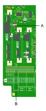
The RS485 interface is used for data transfer to higher-level control systems such as the Process Monitoring system or other systems that support the Wallace & Tiernan RS485 protocol. For more detailed information, please refer to the instruction manual "RS485 interface." You can request this instruction manual from your affiliate or download it from our homepage, www.evoqua.com.
