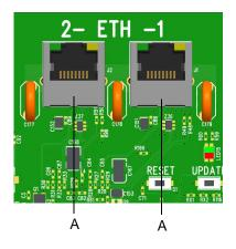
The Blu-Sentinel SE has two integrated Ethernet interfaces (ETH 1 and ETH 2). They are connected internally via an Ethernet switch. The device has an MAC address. The MAC address is displayed in the menu "Settings - Connections - Network." The installed LAN interface allows data visualization via Internet-capable devices and HTTP protocol or standard browser. The LAN interface also supports data communication via the Modbus TCP protocol, see Chapter 4.4 "Modbus TCP interface".
