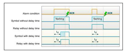
Image 7 Latched alarm with confirmation (acknowledgment option)
