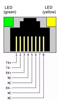
The Ethernet connection is designed in accordance with IEEE 802.3. There are two I8P8C sockets (often referred to as RJ45 sockets) installed. Connection to the HUB or switch can be realized with a 1:1-wire and screened patch cable. Direct connection to a PC network card is possible using a patch cable (1:1) or a crossover cable (crossed network cable). The LEDs are fitted in the 8P8C socket. They display the interface statuses. The meaning of the LEDS is as follows:
