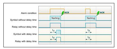
Image 6 Latched alarm with reset acknowledgment option
