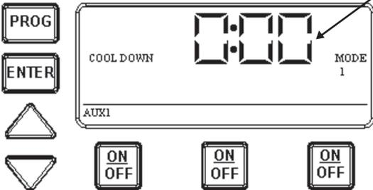
You can override the cool down feature by simply pressing and releasing the ON/OFF key associated with circuit #1. This will end the cool down cycle, and immediately turn off circuit #1.
