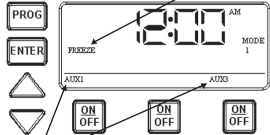
**Aux #1 & #3** will blink indicating the control has activated these two circuits due to a freeze condition. To override the circuits during a freeze condition, simply press and release each of the corresponding ON/OFF keys. This will override the freeze control and turn the devices OFF. The override will only last for one hour, so if the freeze condition still exists after one hour, circuits #1 & #3 will come back on.
