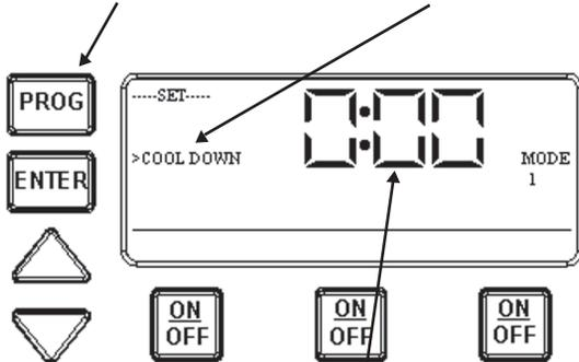
2. The default cool down time is zero. Use the arrow keys to modify the cool down time. The range is zero to fifteen minutes. Use the Enter key or Program key to either save and exit, or save and advance to the next programming feature.
