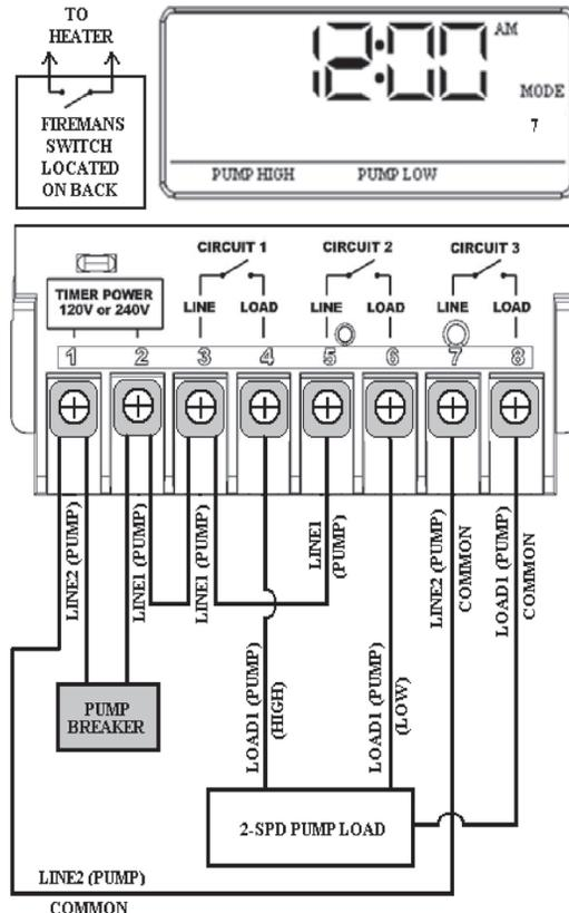
**Mode 6** – (Aux1, Aux2, Aux3) Each of the three single pole circuits are defined generically, and can control any load within each of its individual circuit ratings. All three circuits act independent of each other. The fireman switch closes when circuit one is activated manually by the user and opens when the user manually turns OFF circuit one. The fireman switch remains open when circuit one is activated by a programmed time event.
