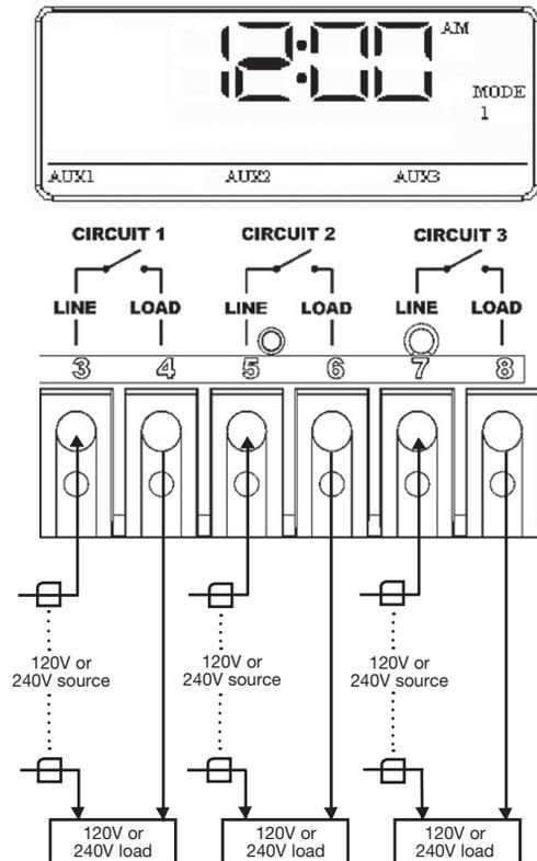
**Mode 2** – (Pump High, Pump Low, Aux3) Circuit one and two are dedicated single pole outputs for a two-speed pump load. Circuits one and two will never be ON at the same time, consistent with a two-speed pump application. Circuit three is single pole circuit for a generic load, and independent of circuits one and two.
