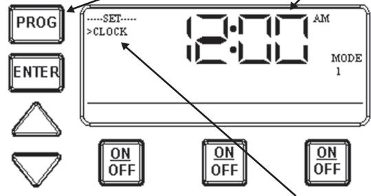
2. After approximately 5 seconds, the **SET CLOCK** will disappear and the display time will stop blinking.
