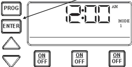
2. After 5 seconds, the display should change to the revision level. The **r1** stands for revision one, **r2** for revision two and so on.
