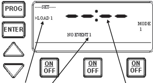
**Circuit #1's first event has not been defined.** You have the ability to program up to three separate events per load or circuit. An event is defined as a complete On and Off cycle.
