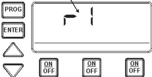
3. Release the **ENTER** key after viewing the revision level. The revision level should disappear and return back to the time of day.
