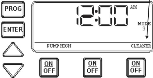
Like the other outputs, the cleaner pump icon is solid after the cleaner pump has turned on. In the event someone manually turns off the filter pump, the cleaner pump will also turn off.
