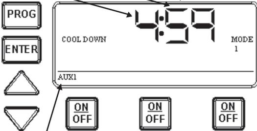
The **AUX1 indicator is blinking** indicating the cool down feature is activated for circuit #1. When the count down display reaches **zero**, the actuated circuits (#1 or #2) depending on mode (2 or 4), will open and the display will change back to the time of day.
