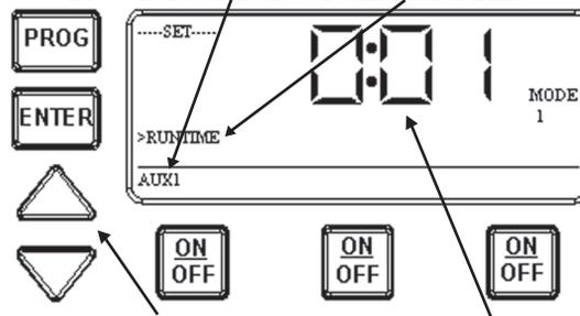
3. Use the **Up/Down keys** to change the **countdown time amount**, in this case 1 minute. Release the ON/OFF key when you have reached the desired countdown time. The circuit will now stay ON for the defined time entered.
