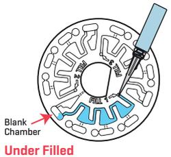
4. Do not introduce air bubbles into the disk. The reagent chambers will not fill entirely and results will be inaccurate. Remove the water sample with the syringe and refill.
