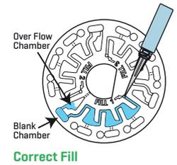
2. Do not overfill the disk. If the disk is overfilled, sample water will flow out of the vent hole in the center of the disk. The disk is not leaking. Dry the disk and run the test.
