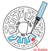
5. Wet disks should be dried thoroughly with a lint free wipe. Handle the disk by the edges. Between tests store the disk on a flat surface. Do not agitate a partially filled disk to avoid leaking and contamination. Partially used disks should be discarded at the end of the day.
