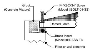
**CAUTION:** The section fitting fasteners must be observed for damage or tampering before each use of the facility and/or at least annually.
