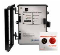
The Compool LX820 controller makes it easy and economical to enhance the safety of commercial spas. In the event of an emergency, pushing the mushroom-style button stops all spa equipment. This action shuts off the filter and up to two jet pumps, while sounding an alarm. Pulling the emergency button back out cancels the alarm, and returns the pumps to normal operation.
