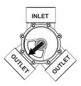
Valve diverter seal position 4
