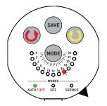
Position 16 (LED on) indicates the diverter partially restricts water flow out of the right side outlet.
