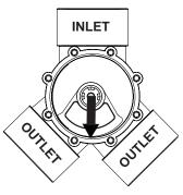
Valve diverter seal position 12
