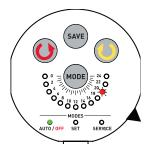
Position 20 (LED on) indicates the diverter restricts water flow for total shut off of the right side outlet.
