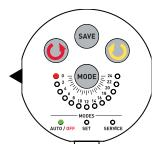
Pposition 0 (LED on) indicates the diverter partially restricts water flow out of the left side outlet. The water flow out of the right side outlet is unrestricted.
