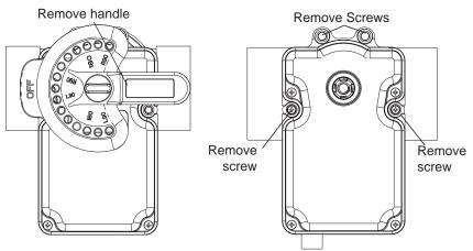
Figure 4. Valve Assembly with Actuator
