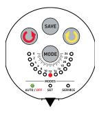
Position 12 (LED on) indicates the diverter partially restricts water flow out of the left and right side valve.
