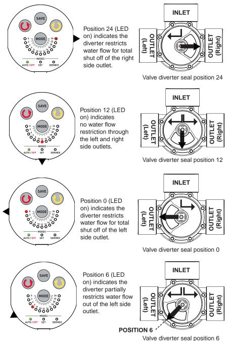
INTELLIVALVE™ Valve Actuator Installation and User's Guide
