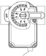
ON1 - ON2 Toggle Switch (Standard valve actuator)
