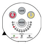
Position 4 (LED on) indicates the diverter restricts water flow for total shut off of the left side outlet.
