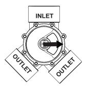
Valve diverter seal position 24
