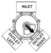
Valve diverter seal position 20
