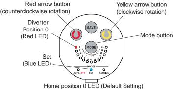
7. **Changing Home Position:** If the current diverter home position which the diverter moved to is not the desired *home* position for the application, simply press and release both the Red and Yellow arrow buttons simultaneously to move the diverter home position to the opposite end point. This is now the diverter home position. For more information see page 11.
