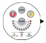
Position 24 (LED on) indicates the diverter partially restricts water flow out of the right side outlet. The water flow out of the left side outlet is unrestricted.
