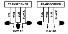
The high voltage wiring section is located behind the service panel in the lower right side compartment. Holes are provided on bottom of enclosure for conduit mounting. The Control can be connected either to 115VAC or 230VAC.
