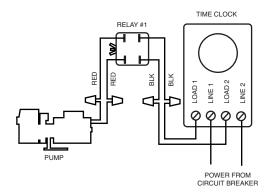
RELAY #1 (plugged into circuit board at **SPA PUMP socket**).
