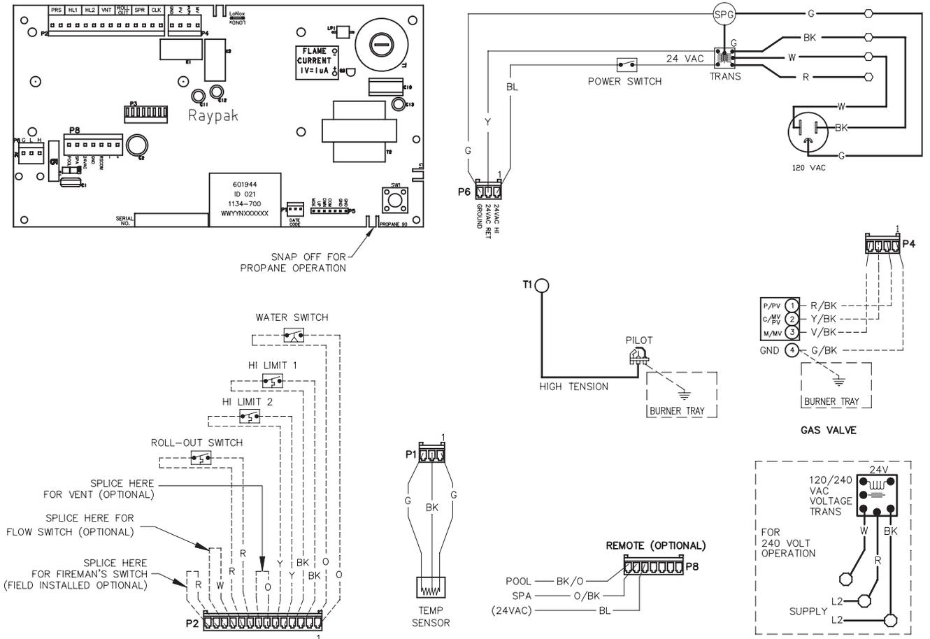
Fig. 20: Wiring Diagram—P156 Only
