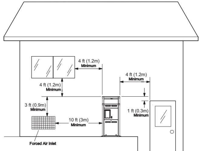
Fig. 5: Outdoor Installation Clearances
