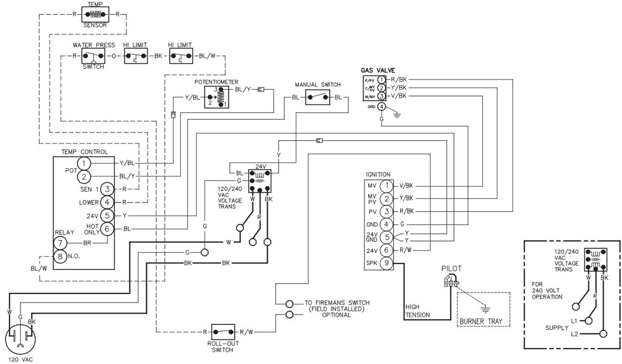
Fig. 19: Wiring Diagram—P106 Only
