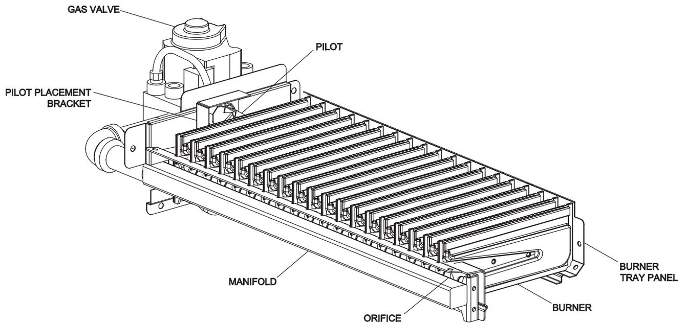
Fig. 26: Burner Tray Assembly
