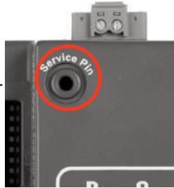
Fig. 22: ProtoNode LER Commissioning Hole Location
