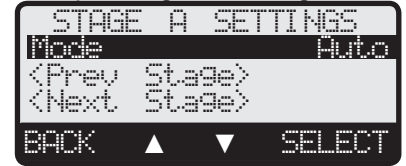
Sequencing Boiler Stage Menu
