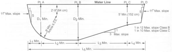
NOTE:  $L_4$  is a minimum dimension to allow sufficient length opposite the board. This may of course be lengthened to form the shallow portion of the pool.  $L_2$ ,  $L_3$ ,  $L_4$  combined represent the minimum distance from the tip of board to pool wall opposite diving equipment.
