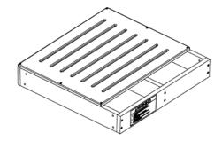
7. Attach part (2) to part (8) using screws (34).
