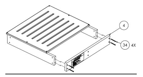
4. Attach part (5) with notch in direction shown to assembly using screws (34).
