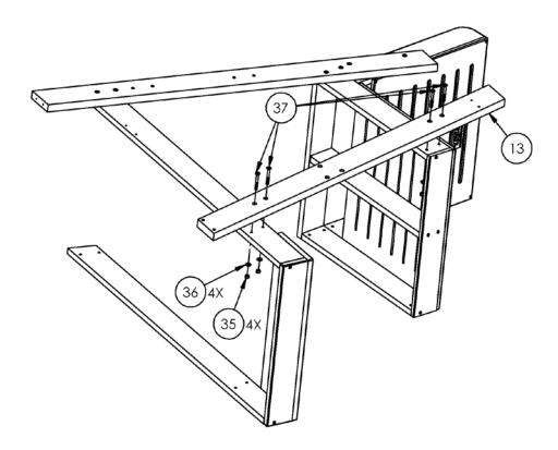
16.Attach step side (23) to assembly using nuts (35), washers (36), and screws (37).
