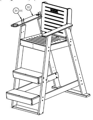
25.Attach braces (24) using screws (34).
