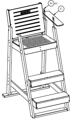
24.Attach arm rest (32) using screws (34).
