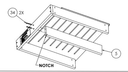
5. Attach part (6) to assembly with screws (34).
