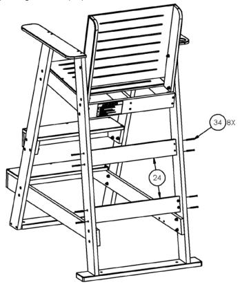
26.Attach cross braces (25 & 26) using nuts (35), washers (36), and screws (33).
