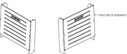
10.Attach part (21) to part (1) using screws (34).
