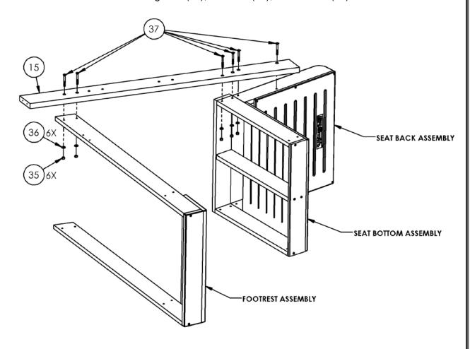
15.Next, attach leg (13) to assembly using nuts (35), washers (36), and screws (37).
