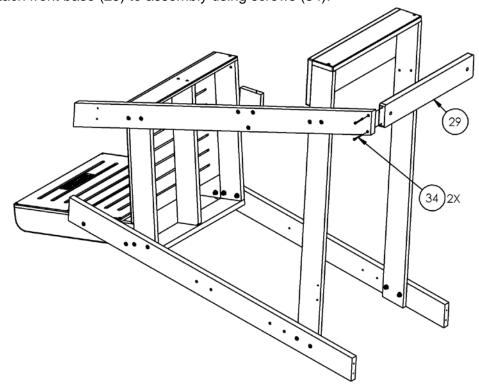
19. Attach leg (14) to assembly with nuts (35), washers (36), and screws (34 & 37).
