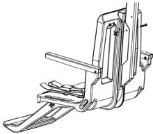
18. Attach foot rest to seat with bolts and thumbnuts.
