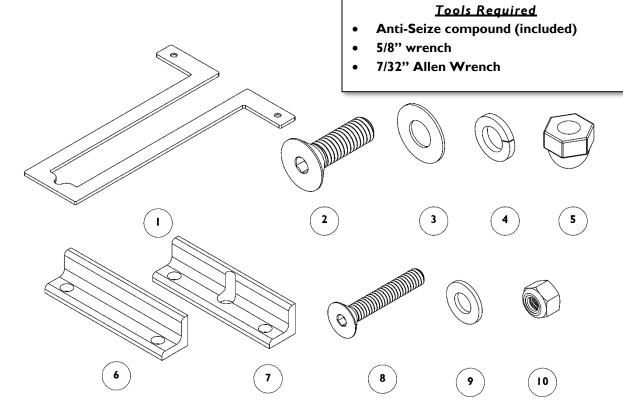
Figure K | Platform Post Mounting Kit Parts
