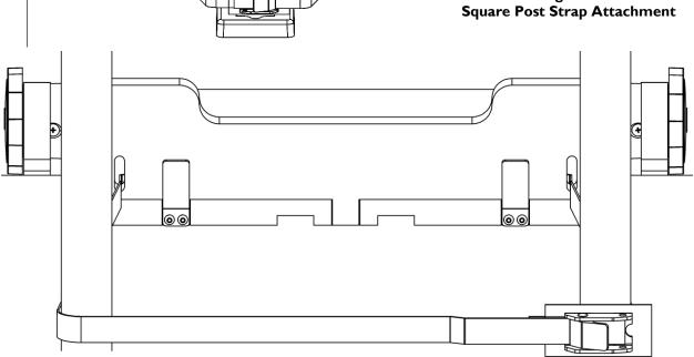
Figure J | Dual Post/Velocity VR Strap Attachment
