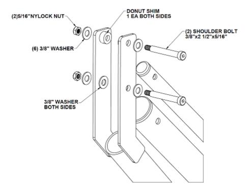
Attach the seat half and the seat belt to the mounting plate of the seat arm using:
