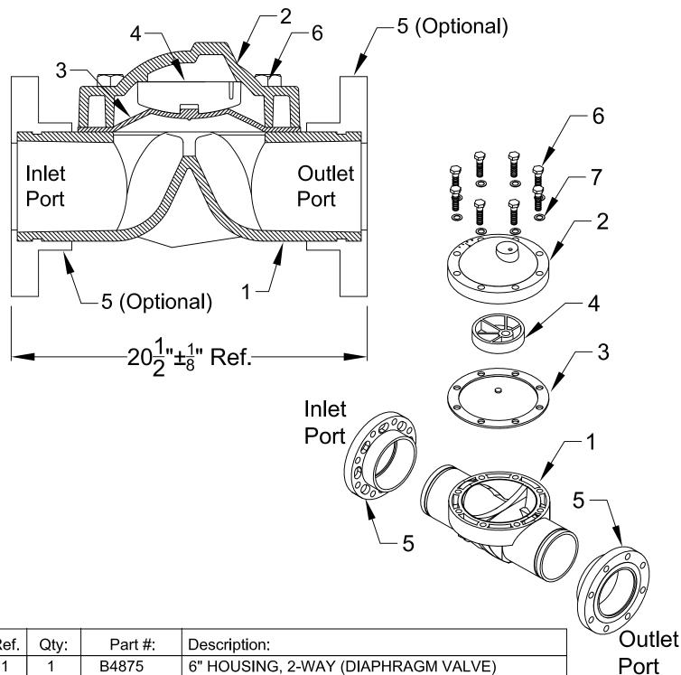
Ref. 6" HOUSING, 2-WAY (DIAPHRAGM VALVE) 1 B4875 1 2 B4762 6" COVER, TAPPED (DIAPHRAGM VALVE) DIAPHRAGM, 6" VALVE, 2-WAY (WITHOUT HOLE) 3 B4763 4 B4878 6" PLATE (DIAPHRAGM VALVE) 5 6" SOCKET FLANGE, SCHEDULE 80 B4815 6 8 94901 HEX HEAD BOLT, 3/4"-10 x 2 3/4" T316L S/S 7 8 94953 WASHER, .765" ID x 1.25" OD, T316L S/S 1/4" NPT x 3/8" OD QUICK ELBOW (NOT SHOWN) 8 B4642
