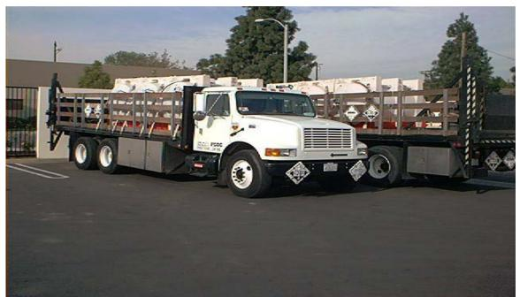
Typical delivery truck. Bulk liquid is pumped from truck to customer's tank via air driven pump. Each delivery is measured and totaled with on-board scale. **Chemical Delivery Bid Specifications**
