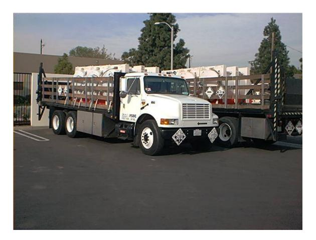
20 Foot Flatbed Tank Truck - 45,000 GVW - Dual Axle Freightliner
