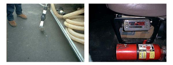
Each style truck is equipped with a PTO that provides power/air to drive a diaphragm pump. Each pump is designed to move material specified. Connections to each type of chemical tank are designed to eliminate cross connection.
